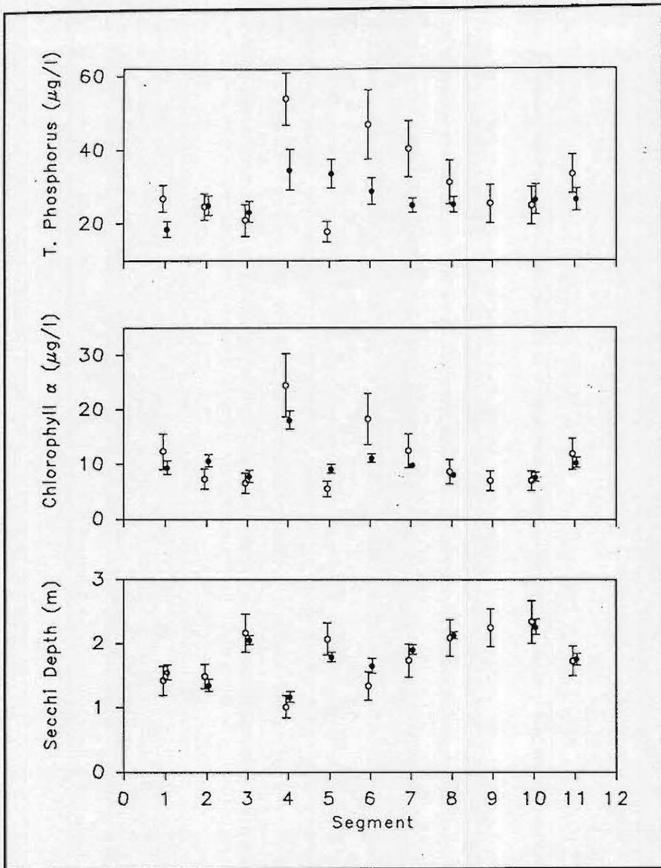
Figure 3. Observed (solid circles) and predicted (open circles) total phosphorus concentrations, chlorophyll a concentrations, and Secchi depths for modeled segments of Allatoona Lake for 1992. Predicted values based on default calibration factors. Vertical bars represent observed and predicted variability. Segment 11 represents the lakewide, weighted average
