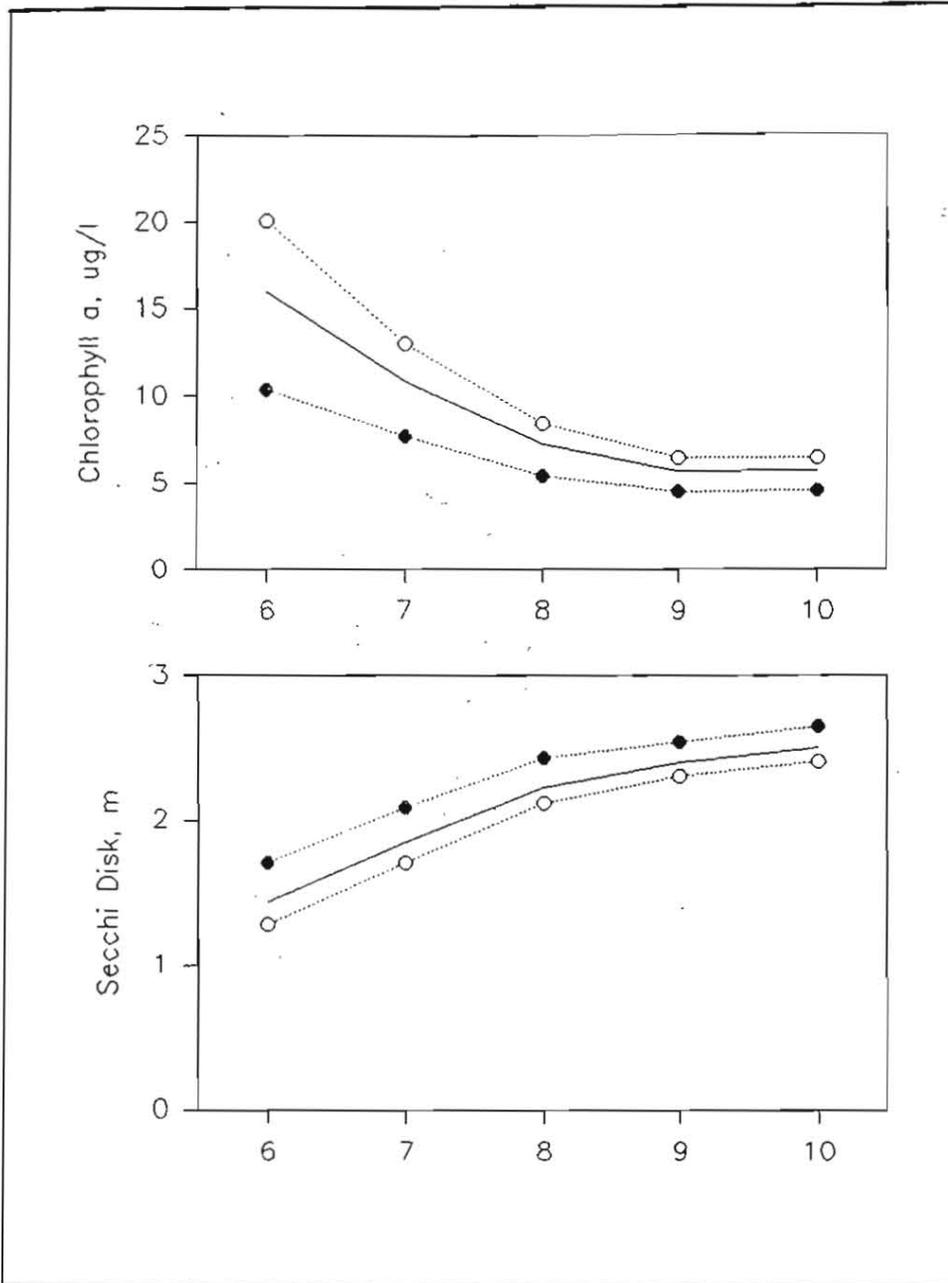
Figure 21. Predicted changes in chlorophyll *a* concentrations (upper) and Secchi depths (lower) in Allatoona Lake associated with changes in inflow nutrient concentration. Predictions for increases of 50 percent (open circles) and decreases of 50 percent (closed circles) are compared with observed data (solid line)
