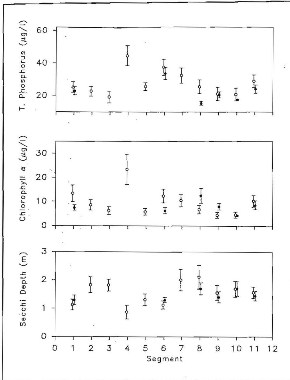
Figure 5. Observed (solid circles) and predicted (open circles) total phosphorus concentrations, chlorophyll a concentrations, and Secchi depths for modeled segments of Allatoona Lake for 1973. Predicted values based on computed calibration factors for 1992. Vertical bars represent observed and predicted variability. Segment 11 represents the lakewide, weighted average
