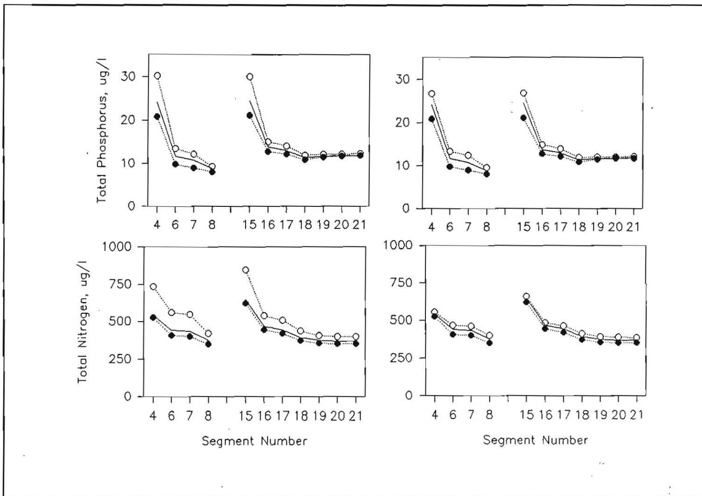
Figure 25. Predicted changes in phosphorus (upper) and nitrogen (lower) concentrations in Lake Sidney Lanier associated with changes in inflow nutrient concentration (left) and inflow volume (right). Predictions for increases of 50 percent (open circles) and decreases of 50 percent (closed circles) are compared with observed data
